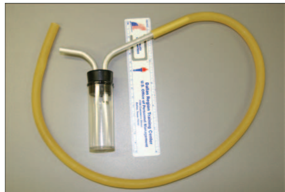
Figure 59. Aspirator used to collect small insects, including Aphthona flea beetle adults. The end of the rubber tube is placed in the mouth; a quick sucking action pulls insects into the metal collecting tube and then into the collecting vial. USDA-APHIS.
