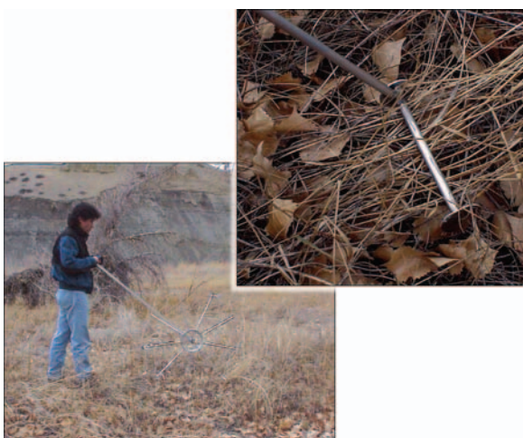
Figure 82. Wheel sampler used in vegetation monitoring. AAFC.
