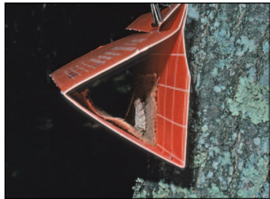
Figure 5. Modified delta trap used as a mating station for monitor adult females.
