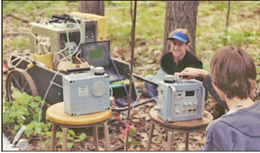
Figure 42. Co-located SF 6 detector and portable electroantennogram sensor used to verify that the tracer gas, SF 6 , is a realistic model for the movement of dispartlure in a hardwood forest.
