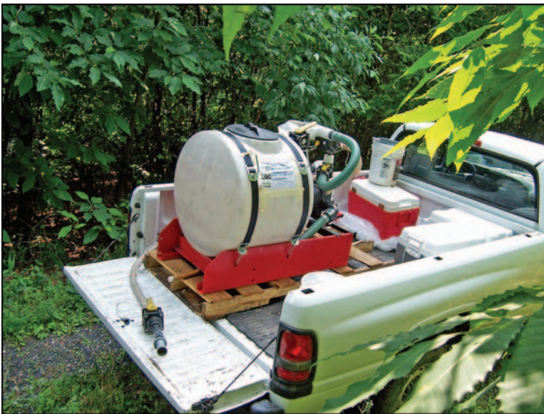
Figure 56. Modified hydroseeder used to apply a tank mix containing Disrupt II flakes to individual trees.
