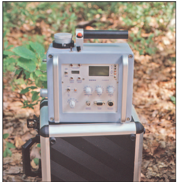
Figure 23. Portable electroantennogram sensor supplied by Jan van der Pers to measure atmospheric pheromone concentration in areas treated with Disrupt II flakes.
