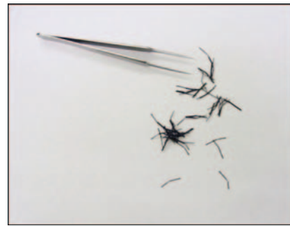
Figure 40. Scentry hollow fiber dispensers containing racemic disparlure.
