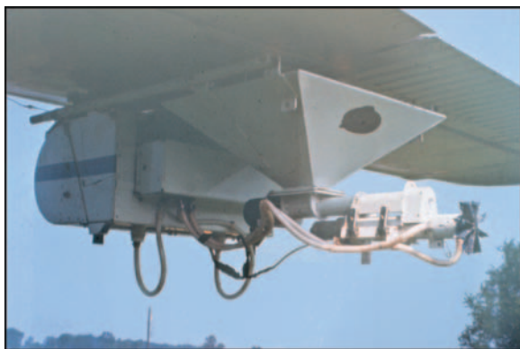
Figure 1. Specialized application equipment mounted under the wing of a Cessna 206 for dispensing the flake formulation of racemic disparlure (Disrupt II).
