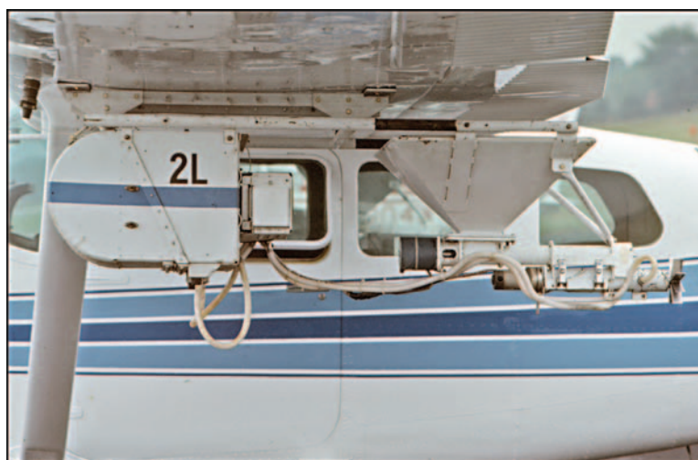
Figure 2. Flakes and sticker are mixed in a chamber then dispensed through a spinner.
