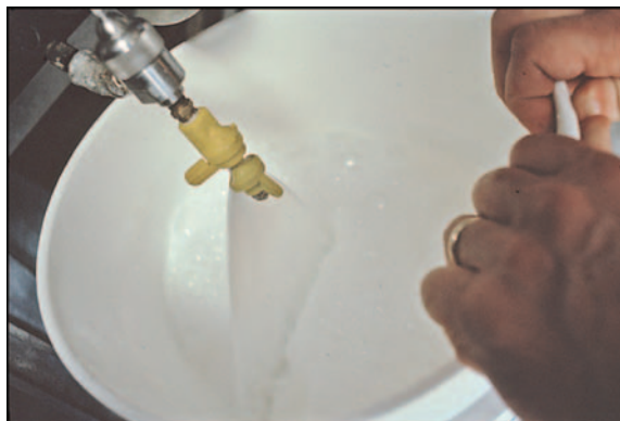
Figure 9. CP nozzle with check valve used to apply bead formulation of racemic disparlure.
