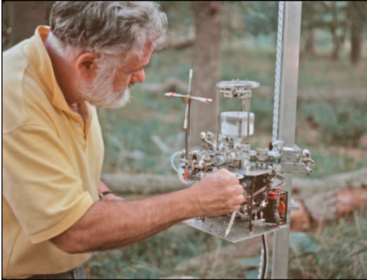
Figure 21. Dr. Uwe Koch and his portable electroantennogram sensor, used to measure atmospheric pheromone concentration in plots treated with disparlure.
