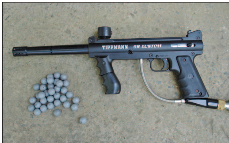
Figure 58. Paintball guns and paintballs loaded with a SPLAT formulation of racemic disparlure for ground-based application for gypsy moth mating disruption.
