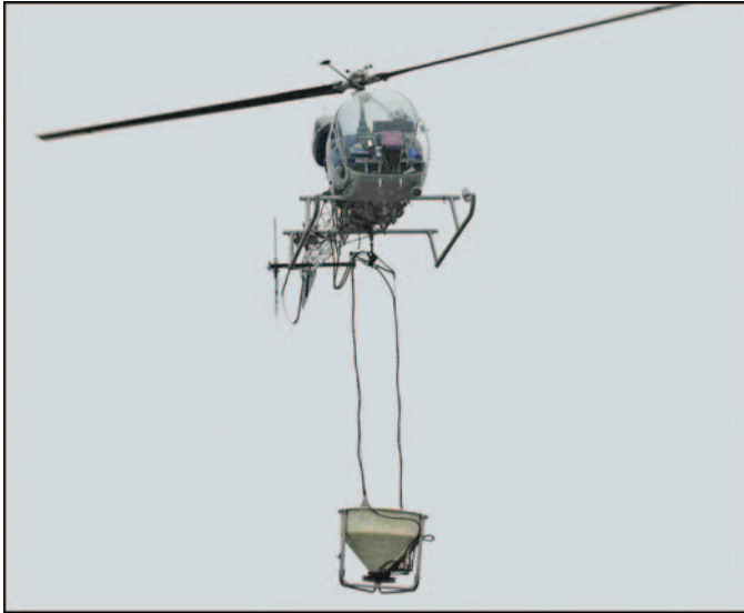
Figure 39. Fertilizer spreader modified to apply mating disruption formulations by helicopter.
