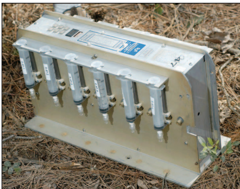
Figure 26. One of a series of syringe samplers used to collect air samples containing a tracer gas to model the movement and distribution of pheromone in a hardwood forest.
