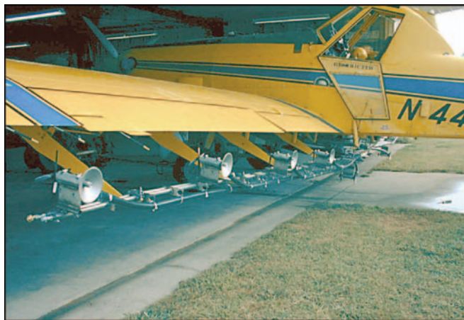
Figure 20. New flake dispersal system (Prototype II) installed on Air Tractor 402. Flakes were dispensed onto a rotating cone attached to a wind-driven propeller and coated with sticker emitted from flat fan nozzles.
