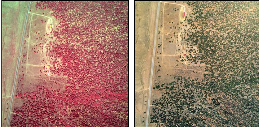
Figure 6. CIR and true-color photography, pinyon pine mortality, Grand Junction, CO (Paul Ishikawa). Airborne sensor: Proback digital camera, 35 mm.
