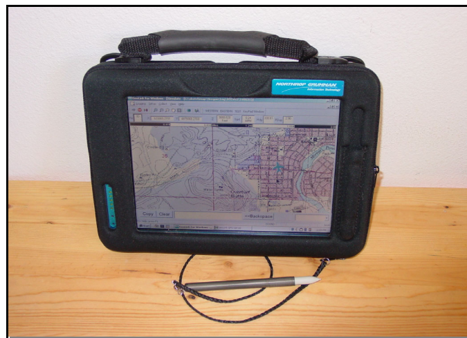
Figure 14—The HammerHead 3 from Walkabout Computers, Inc. The PC and transfective active touchscreen display are integrated into the rugged housing.
