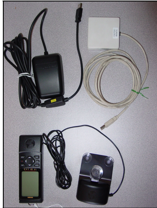
Figure 9—GPS receivers used include USB units ( top ) and the Garmin 12XL with antenna ( bottom ).
