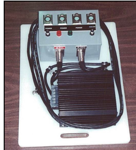
Figure 7—Custom power distribution boards were developed by FHTET for powering the system using the aircraft's electrical system.
