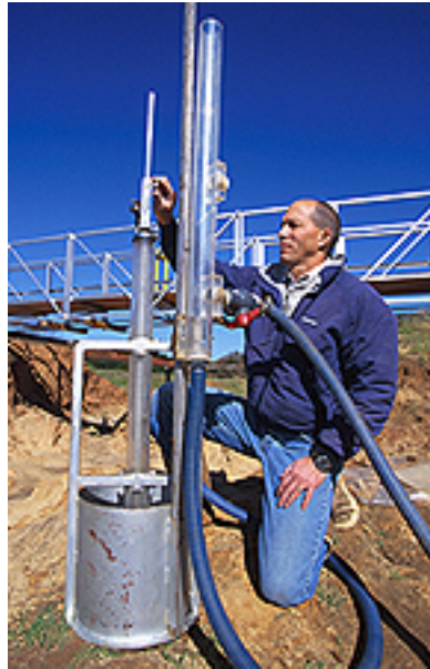
The jet test developed by ARS for measurement of soil erodibility is an ASTM standard.
