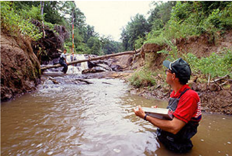
Observing changes in channel geometry and stream corridor habitats caused by water rushing over a headcut.
