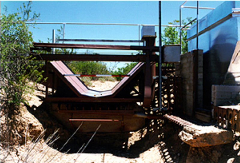
A runoff-measuring flume with a traversing slot sediment sampler.
