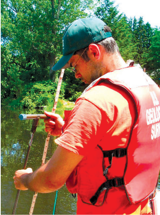
Figure 2. A probe is used to collect data for a map of sediment thickness and extent.
