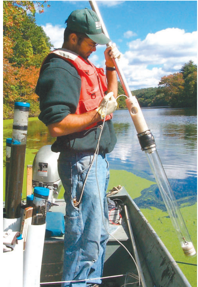
Figure 3. A piston corer is prepared for collection of a sediment core.
