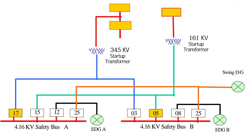
AC Power Distribution System with Y Connection to Safety Buses
