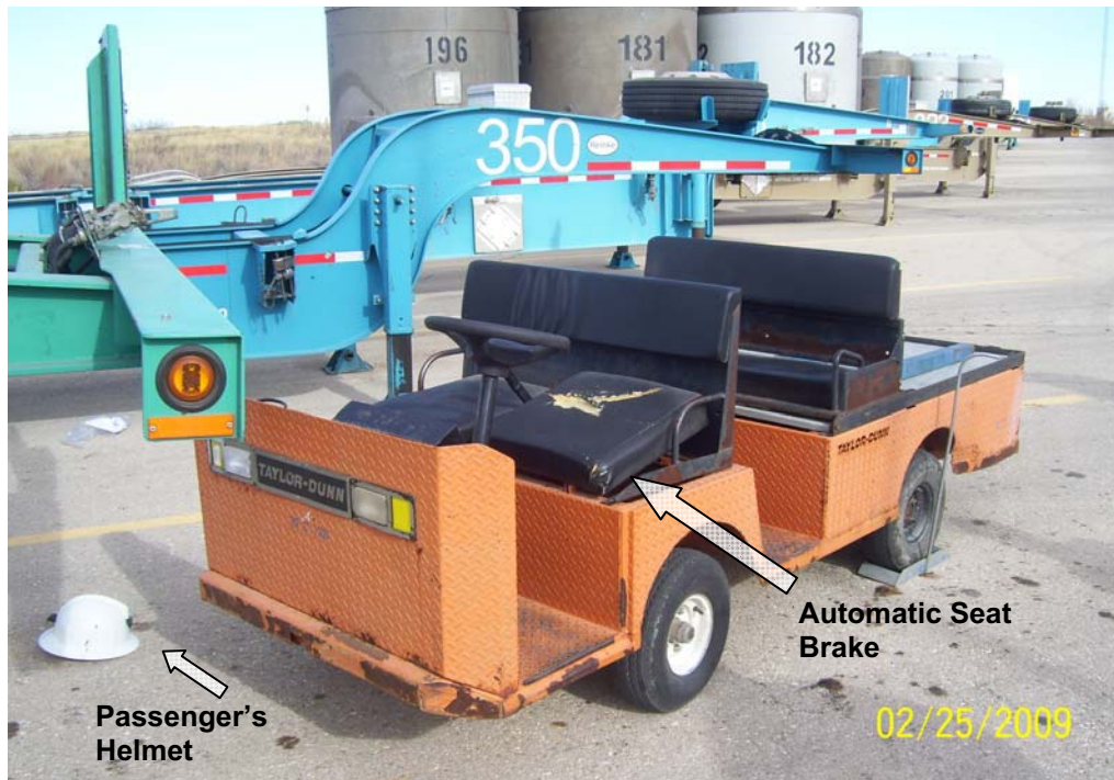
Figure 7: Taylor-Dunn Cart Involved in Accident (showing angle related to trailer)
