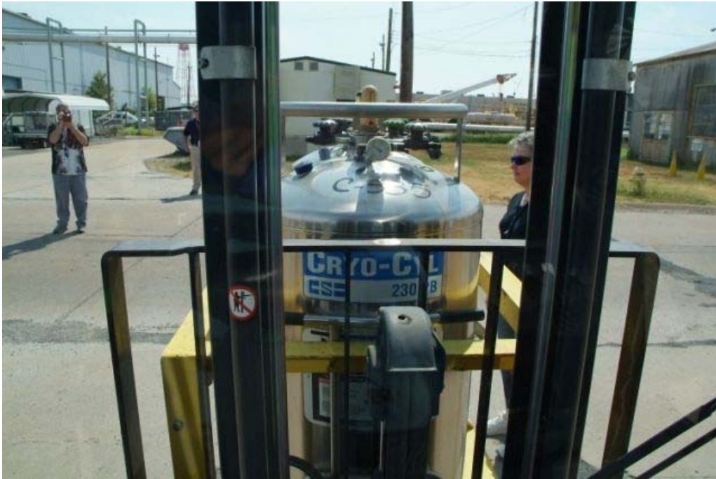
Figure 2.3-5. View in the Direction of Travel, Obscured by the Dewars and Mast Pillars
