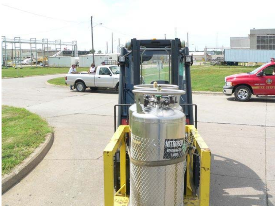
Figure 2.3-4. Front View of Forklift Showing Mast Pillars and Roll Cage Post
