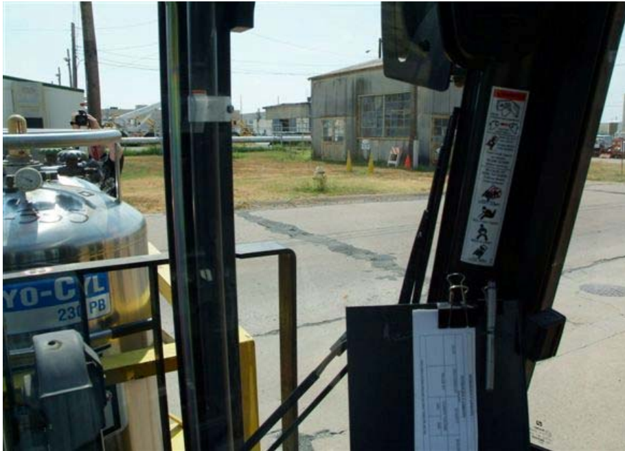
Figure 2.3-3. Inside the Forklift Cab Showing Field of View Impairment From the Windshield Wiper, the Post, and Door Frame
