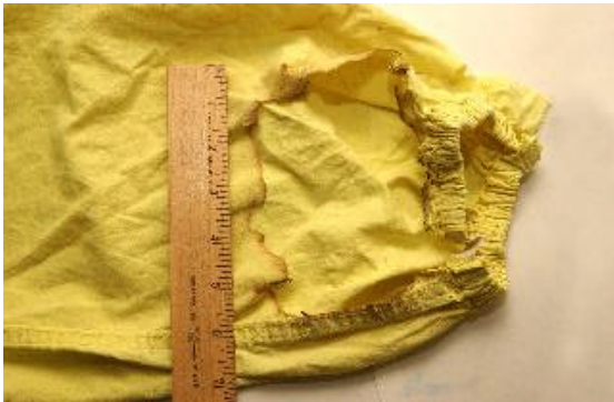
Figure 6. Burned PPE - Anti-C Pant Leg
