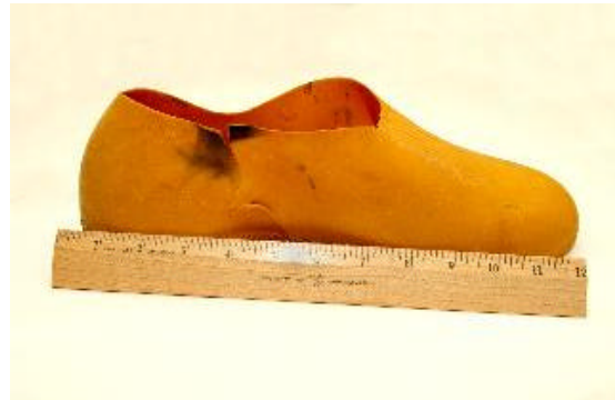
Figure 7. Burned PPE - Shoe Scuff
