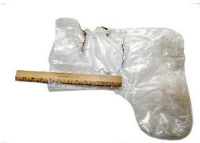
Figure 5. Burned PPE - Clear Plastic Bootie
