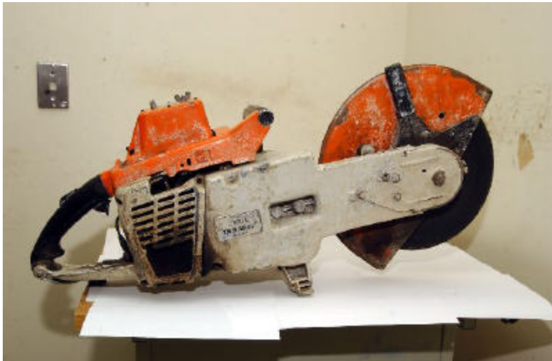
Figure 2. Stihl Cut-Off Machine
