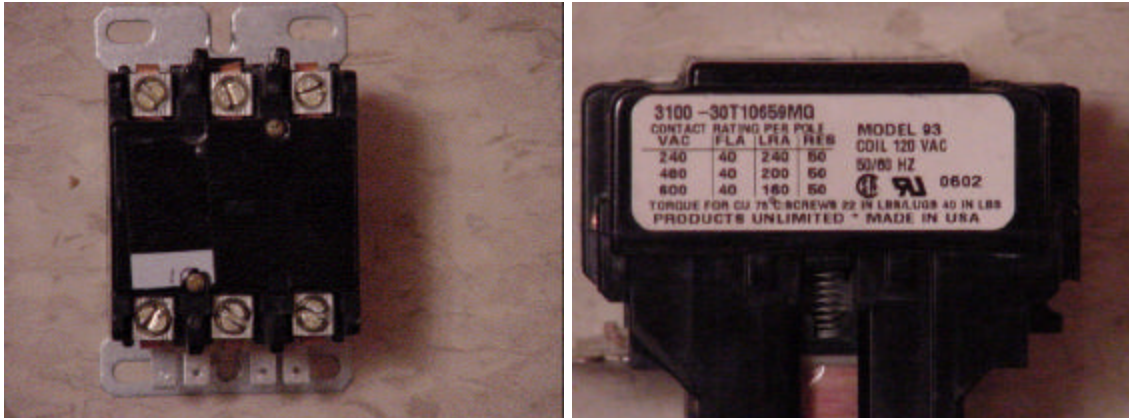
Exhibit 13. Contactors Used by Precision Boilers, Inc.
