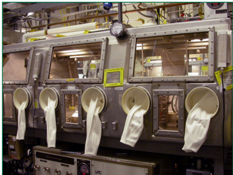
Exhibit 2.3-1 Glovebox G138, where the uranium nitride pellets were loaded into the Swagelok® couplings.
