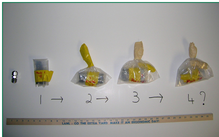
Exhibit 2.3-2 A simulation of the sequence of packaging the Swageloks® in plastic bags. It was later determined by LANL that only three bags were used.
