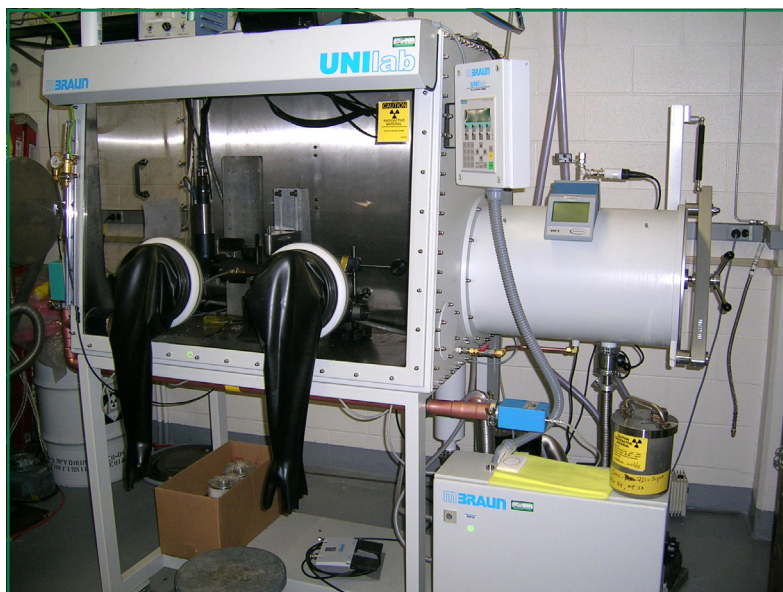
Exhibit 2.6-2 The laser-welding glovebox in room R3 as found during initial re-entries by LANL. The chamber on the end of the glovebox is the antechamber through which items are passed in and out of the box.
