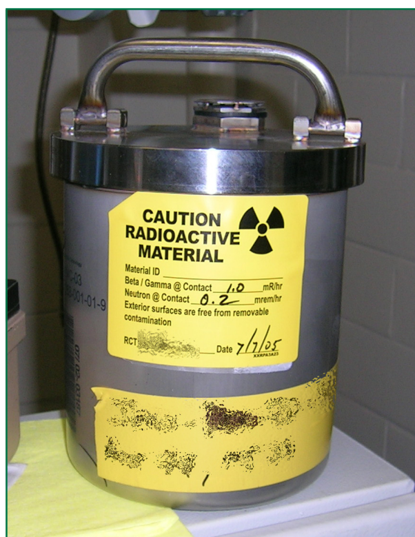
Exhibit 2.3-3 The Hagen can that was used for transferring the uranium nitride pellets from PF-4 to Sigma.
