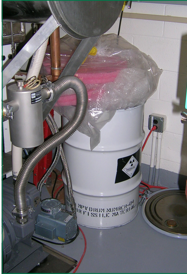
Exhibit 2.3-4 The Type A shipping drum and packing material that was used to transfer the uranium nitride pellets to Sigma. The drum was found in room R3 behind glovebox 2.
