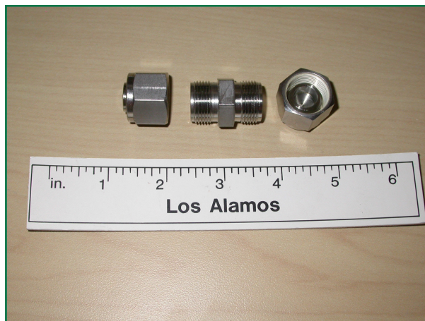
Exhibit 2.1-2 The uranium nitride pellets were contained within Swagelok® couplings and sealed with end caps to maintain an inert atmosphere.
