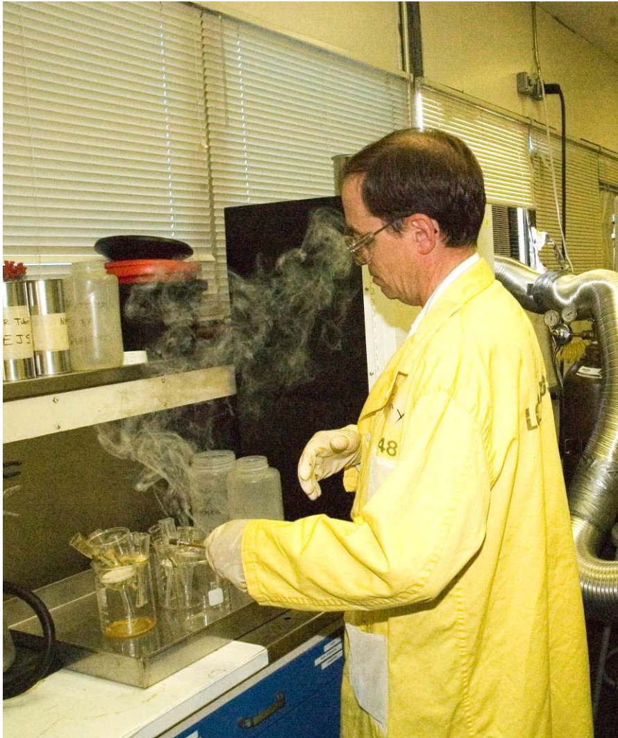
Figure C-9 The concentration of the irritant smoke at some points during the smoke tests was strong enough to cause the Technical Liaison to pull back from the work area. When the Technical Liaison took certain postures likely to have been taken by workers, the released smoke would pass through the breathing zone before being re-circulated to the work area by the eddy current.
