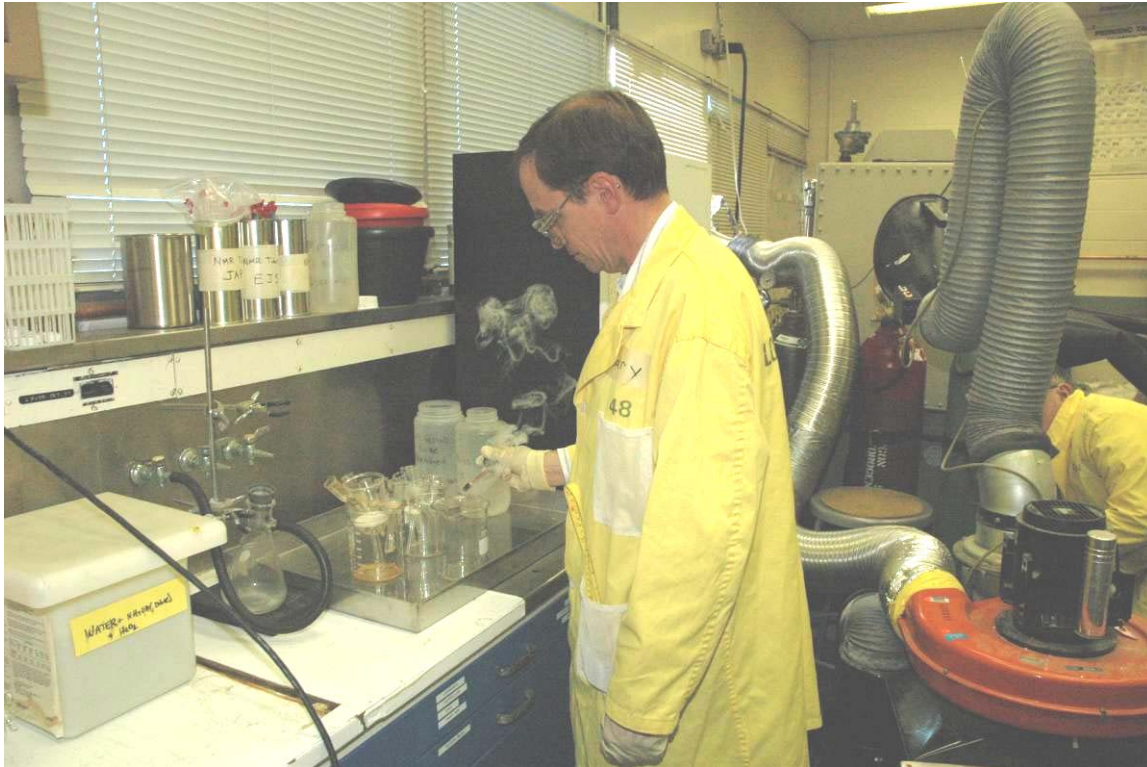
Figure C-5 The Technical Liaison performing the smoke tests stood upright at point A (see Figure C-1) and released smoke at the top of the beaker that would have been used to mix the aqua regia. The released smoke traveled slowly two to three feet to the right of the IH as it began to rise steeply. It initially appeared that the air currents were traveling away from a worker standing at point A. However, when the smoke reached approximately seven to eight feet height above the floor it curved back to the left and began to descend down toward the work area and into the breathing zone of the Technical Liaison. The Technical Liaison could smell and taste the irritant smoke as it descended. The smoke tended to stay in a plane parallel to the wall, with only minimal diffusion toward the center of the room. This apparent eddy current in the air flow patterns at the bench top was stable. Repeated smoke tests yielded similar results.
