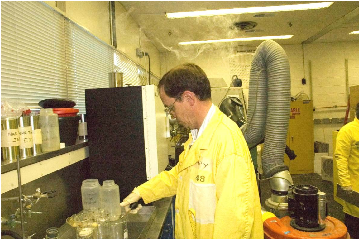
Figure C-6 Smoke entrained in the eddy current descending back down into the breathing zone of the Technical Liaison.
