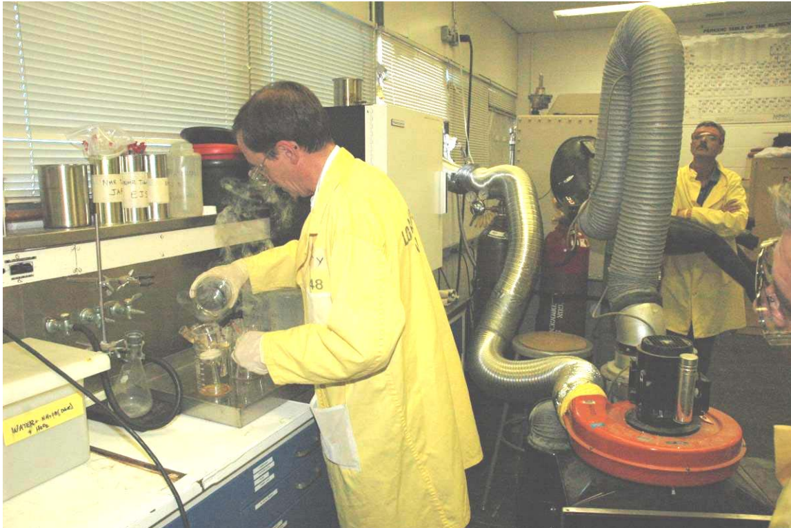
Figure C-8 The Technical Liaison releasing smoke at the top of the beakers containing Büchner funnels (“frits”) while holding a beaker in his right and leaning slightly forward to be better able to observe the frits. A similar posture was likely to have been taken by a worker during the event. With the Technical Liaison in this position a “chimney effect” was observed. Smoke released at the top of the beakers could be observed traveling up along the surface of the Technical Liaison’s right arm and/or along his chest and into his breathing zone.
