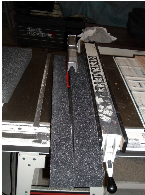
Figure 4. ETHAFOAM 900® Fits Under the Blade Guard Assembly.
