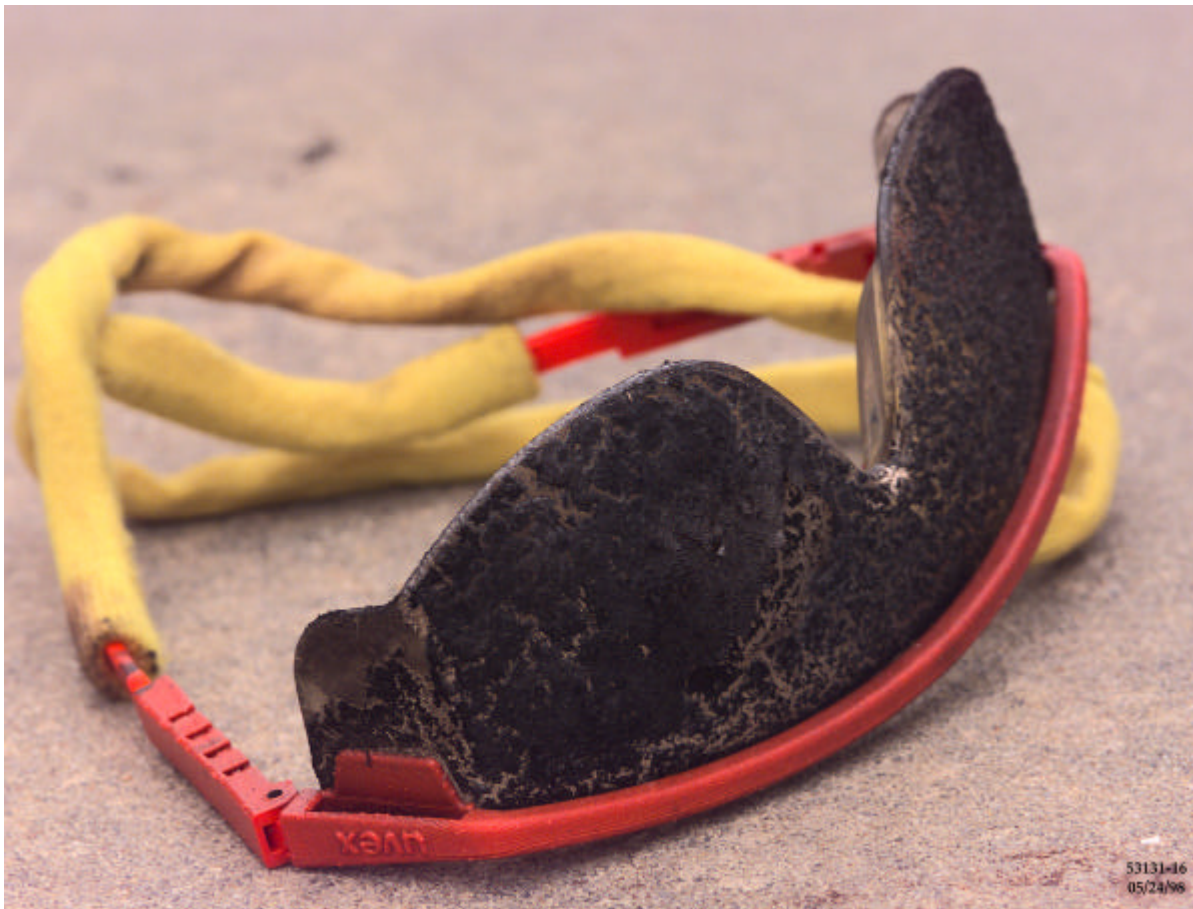
Figure 2-6: Safety Glasses Worn by Electrician #1
