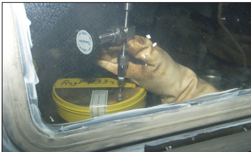
Exhibit 2-6 shows the head gas sample being taken on one of the packages.
