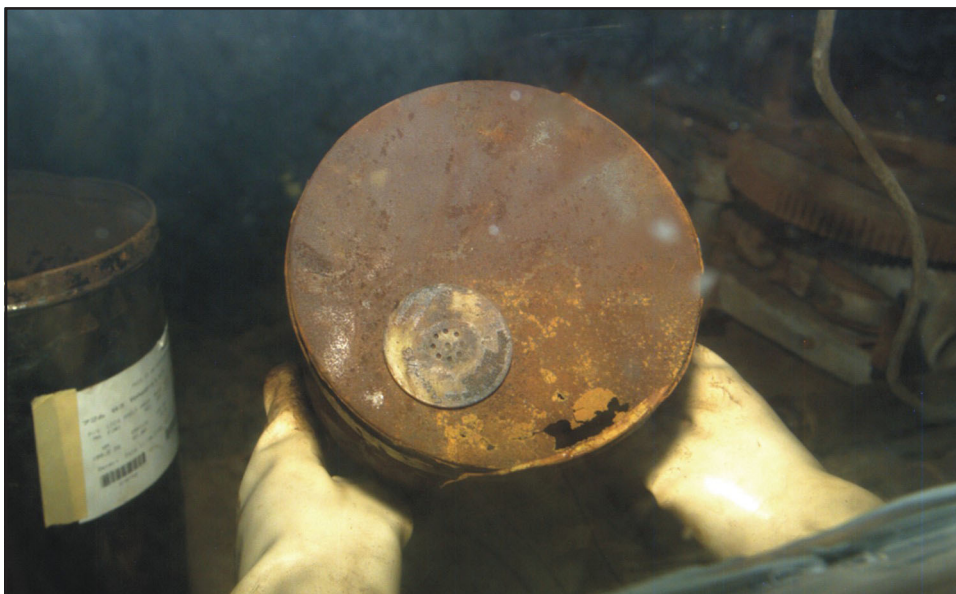
Exhibit 2-10 shows the inner can lid failure of P1.
