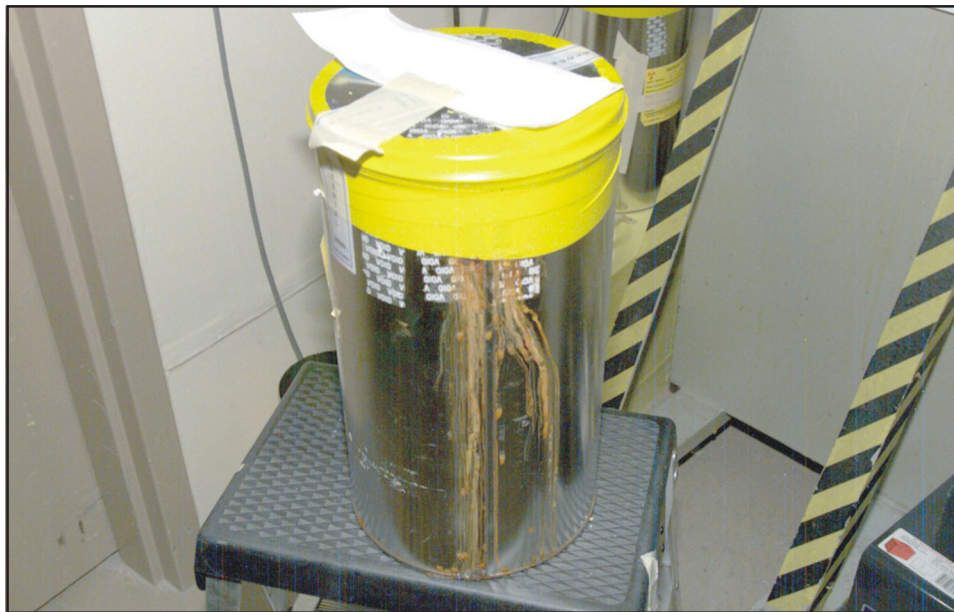
Exhibit 3-5 shows a package with apparent corrosion products seeping down the side of the package.
