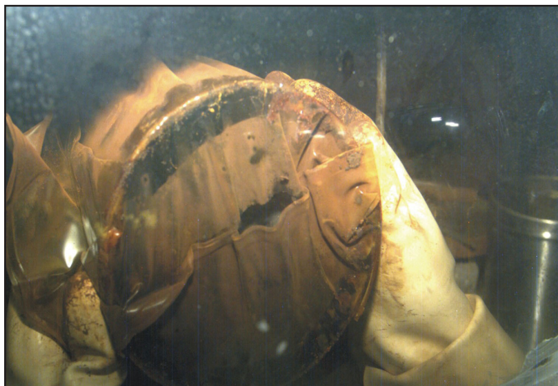
Exhibit 2-8 shows the bag failure of P3.
