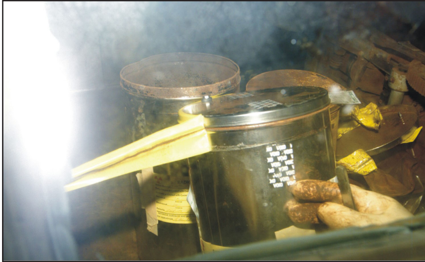
Exhibit 2-7 shows the rust on the tape and under the lid of the outer can.
