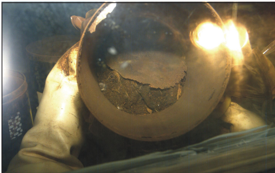
Exhibit 2-11 shows the inner can failure of P3. Note that this view is from the bottom of the can
