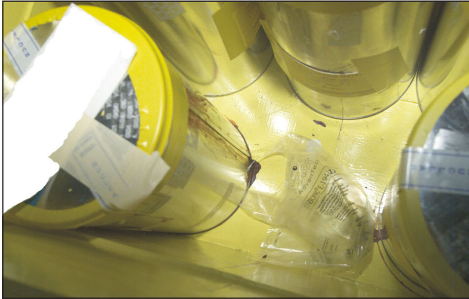
Exhibit 3-3 shows the corrosion products seeping down a package and onto the cart.
