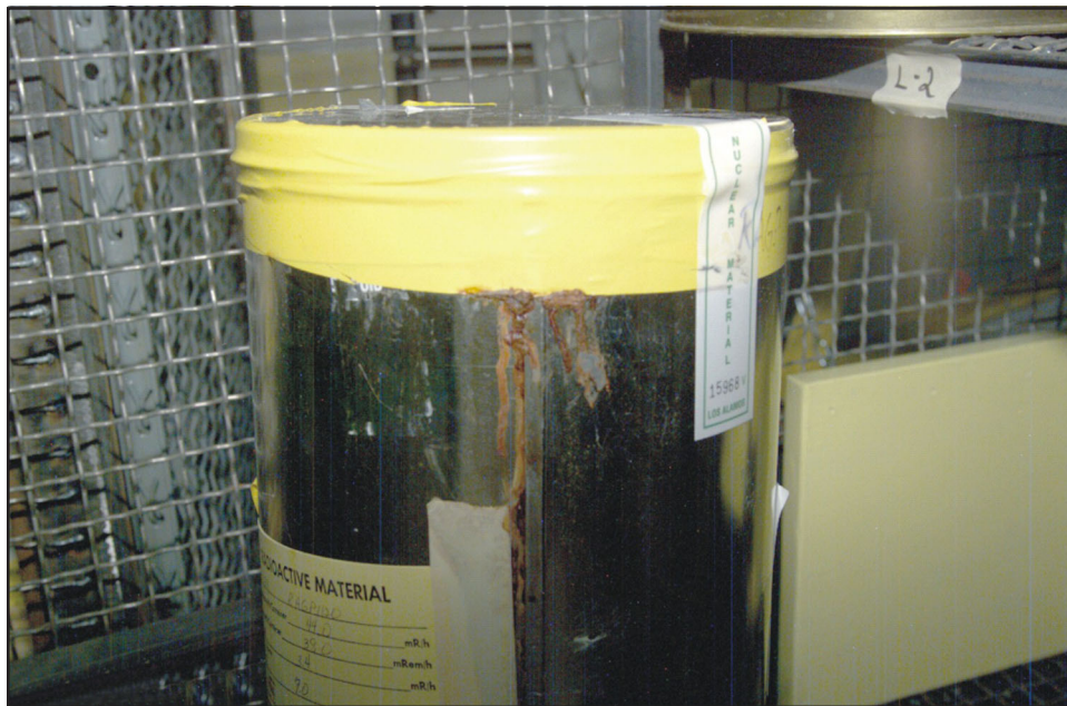
Exhibit 3-4 shows a package with apparent corrosion products seeping under the taped lid.
