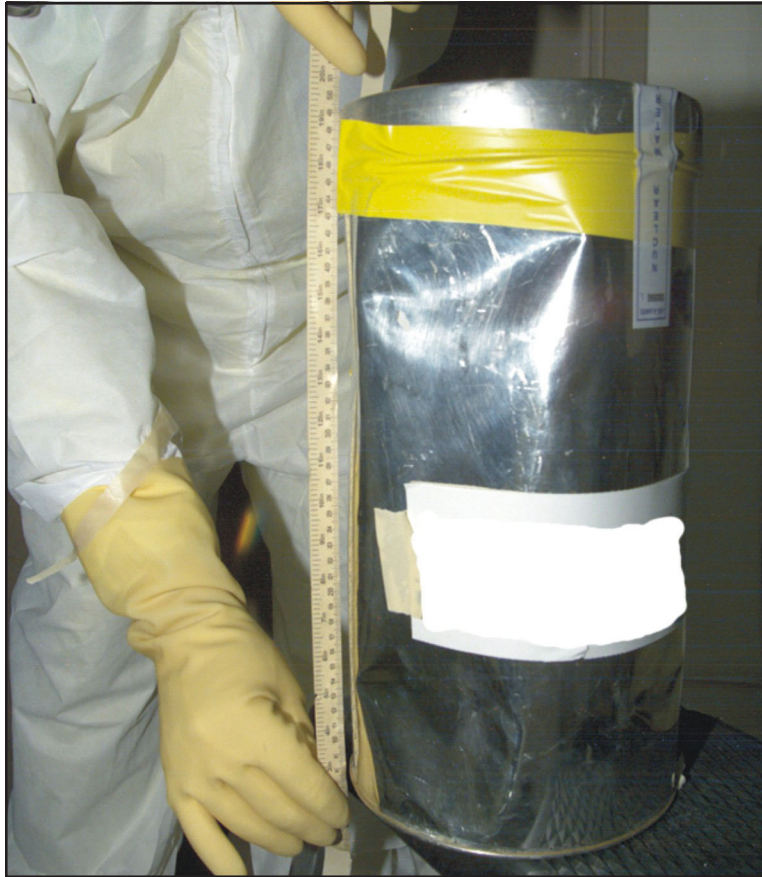
Exhibit 3-7 shows the side of a suspect “paneled” package.
