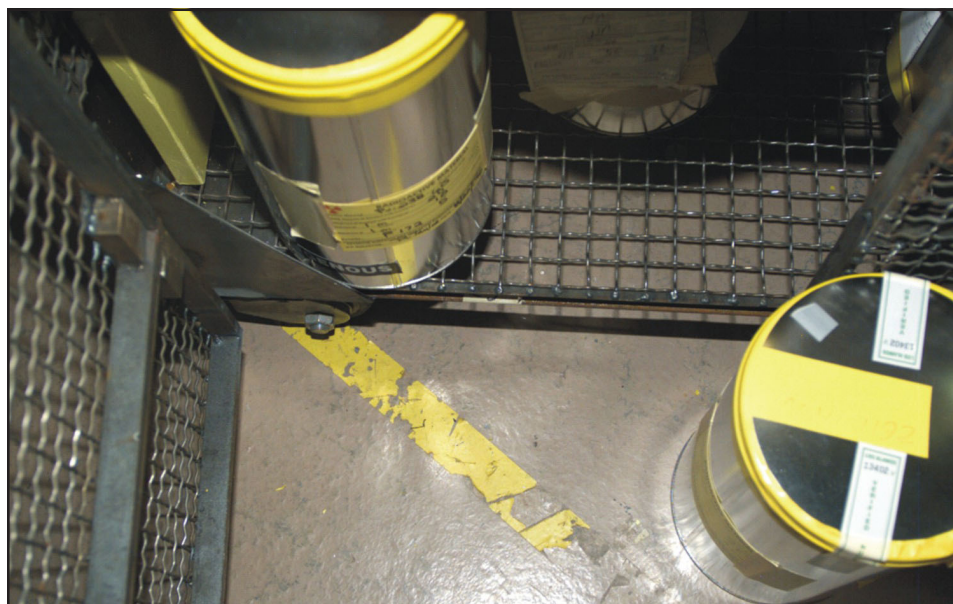
Exhibit 2-4 shows a package on the floor and a suspect package in the cage directly in front of the hot spot location. Note the position of the sidewall seam on the suspect can.
