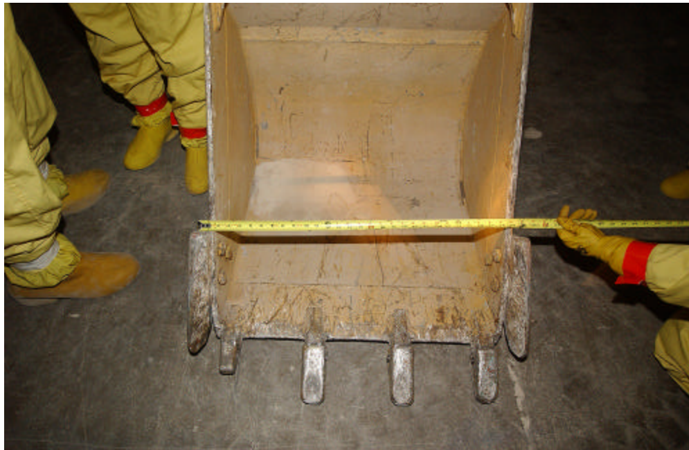
Exhibit 2-8. Trackhoe Bucket Attachment (30 Inches in Width, 4 Teeth Spaced Approximately 8 Inches Apart)
