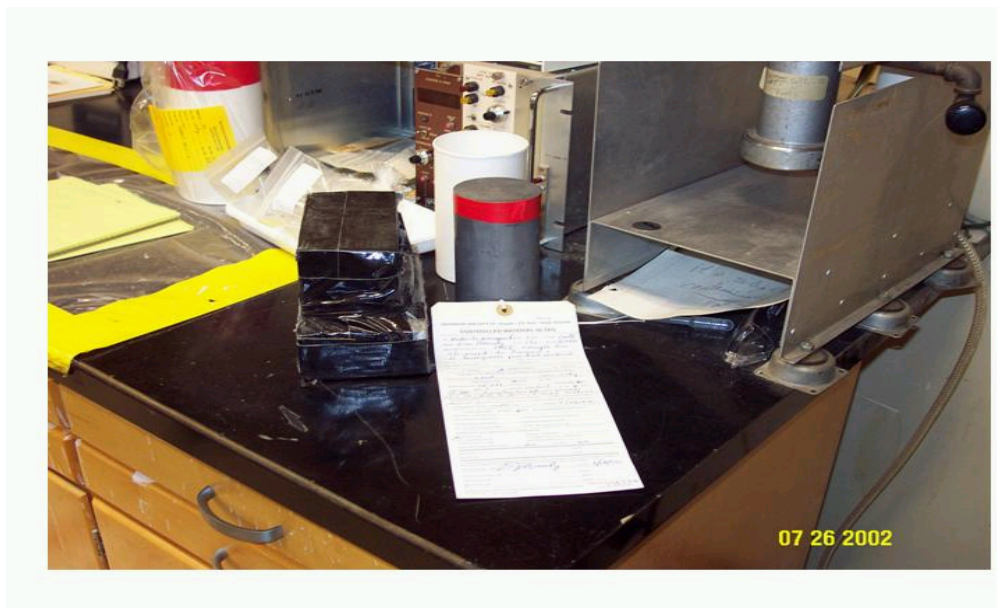
Figure 7. Lead pig containing 11 mg Cf-249 source.
