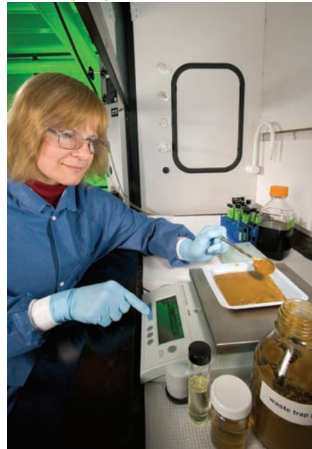
Biologist Karen Scott prepares a sample of trap grease for conversion to biodiesel. In the foreground are samples of distilled (left) and crude (center) biodiesel from trap grease.
