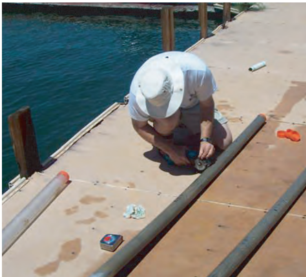
Figure 6. Preparation of polycarbonate core tube liner for transport to laboratory.
