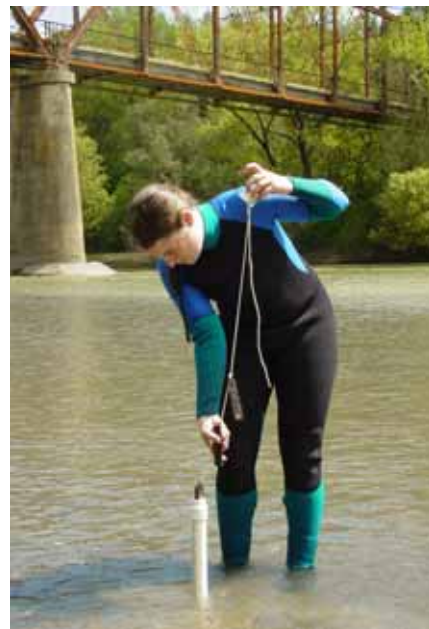
Figure 8. Installation of a piezometer 1 to 2 m into the streambed and placement of temperature loggers into a nearby piezometer
