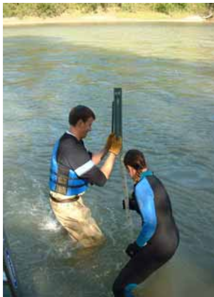
Figure 8. Installation of a piezometer 1 to 2 m into the streambed and placement of temperature loggers into a nearby piezometer
