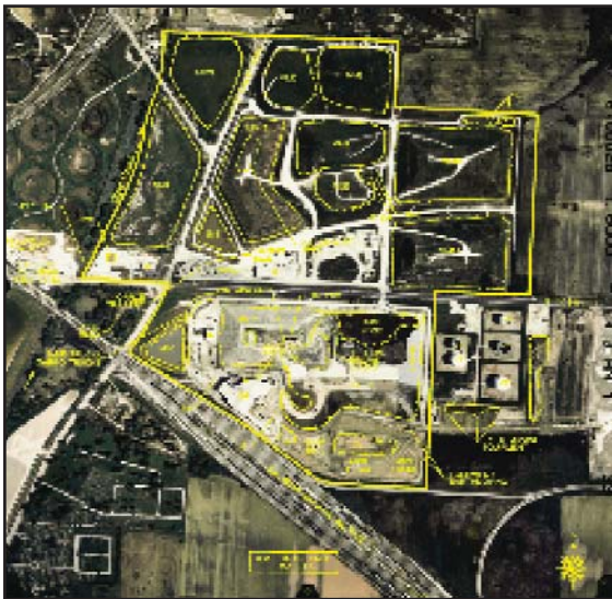
Figure 1. Image is a 1957 aerial photograph which reveals disposal operations located at the center of the site. A large impoundment, excavated areas and active disposal areas are visible. As the significant features and disposal activity are traced through time with eight subsequent sets of photographs, the active area within the site becomes larger in extent.
