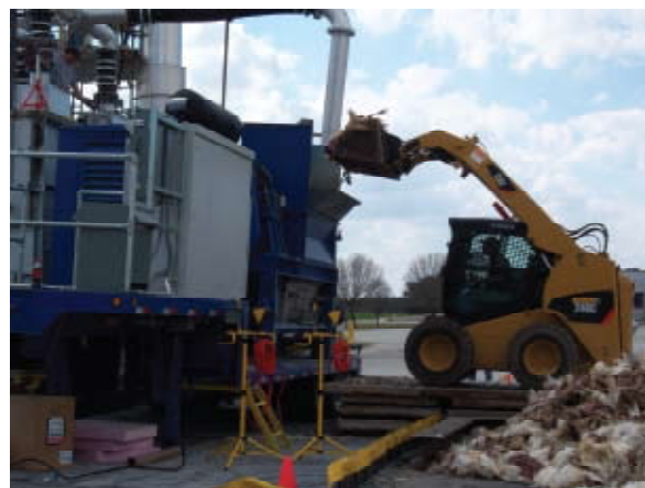
Figure 2-6. Feeding Animal Carcasses into Macerator
