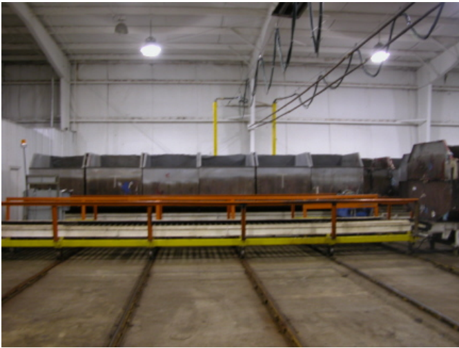
Photo 19. Autoclave Bins on Transfer Cart
