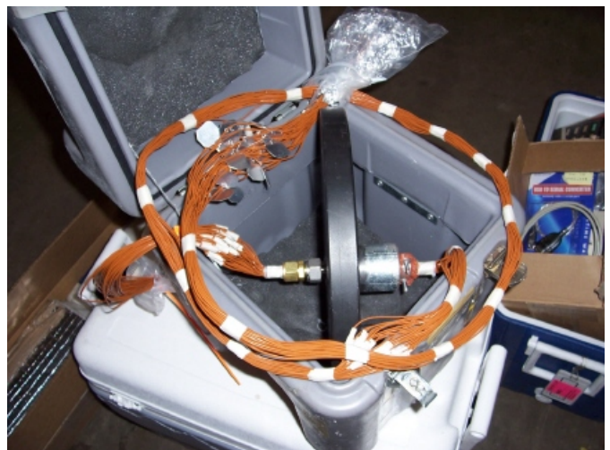
Photo 22. Fabricated Flange Port to Allow Thermocouple Wires to Pass Through
