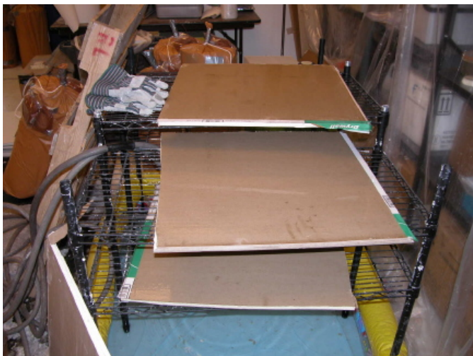
Photo 5. Wallboard on Dry Rack
