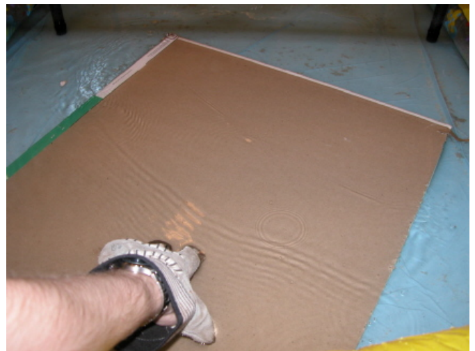
Photo 4. Submersing Wallboard Sheets
