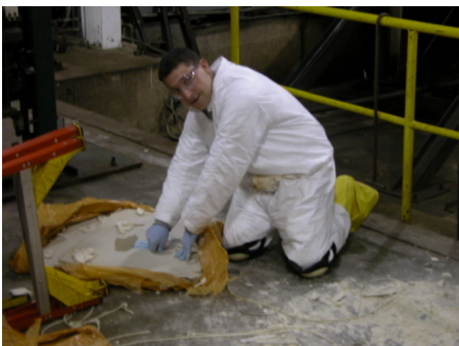
Photo 41. Removing BI Test Pouches from BDR
