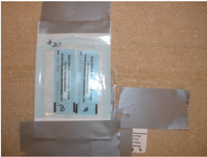
Photo 7. Sample Point (Thermocouple Paired with a BI Test Pouch)
