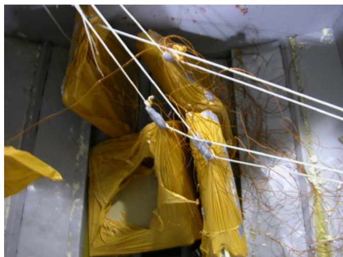
Photo 36. Vertical Packaging Orientation After Autoclaving
