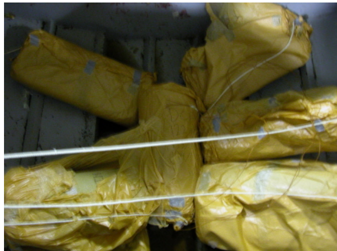
Photo 32. Loose Pack Carpet Bin After Autoclaving
