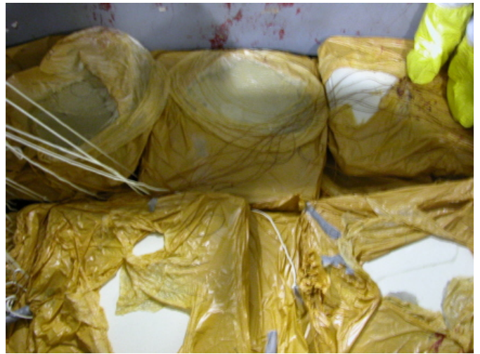
Photo 28. Wallboard Bags After Autoclaving
