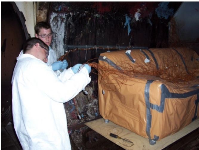
Photo 39. Connecting Thermocouple Wires
