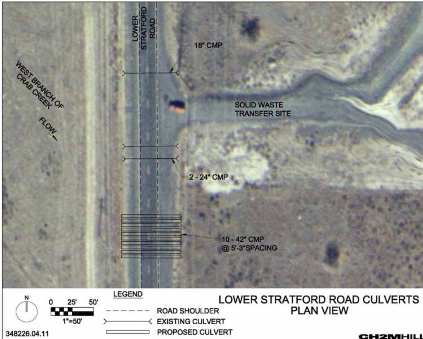
FIGURE 20 Lower Stratford Road Culverts Plan View
