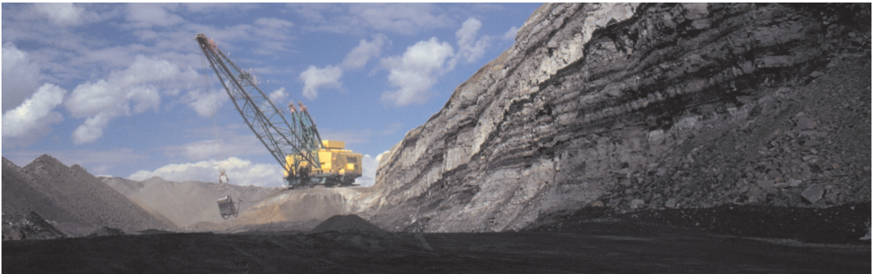
Figure 27A. Modern strip mine: Dragline in pit at Peabody-Western's Black Mesa mine located in the Navajo-Hopi joint-use area in Arizona.
