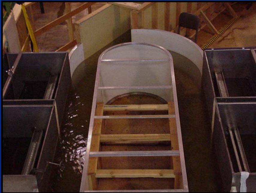
Scale model holding tank for separated fish
