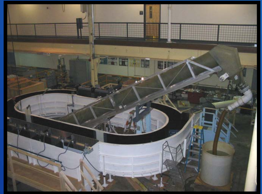
Prototype holding tank For separated fish
