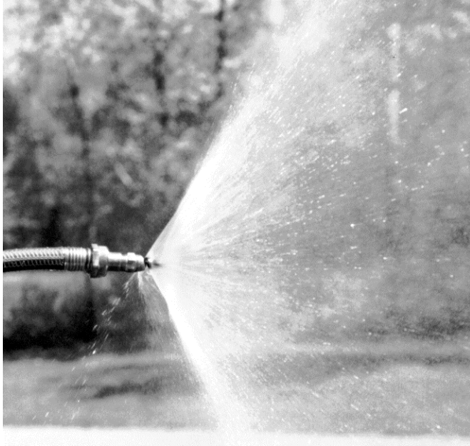
Figure 2-1 – Spray Aeration nozzle spraying water at 0.5 L/s (8 gpm)
