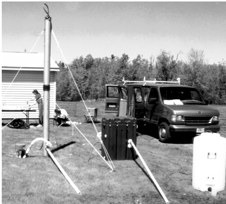
Figure 2-2 –Aeration Systems (bubble - center; Tower - left; spray - right)
