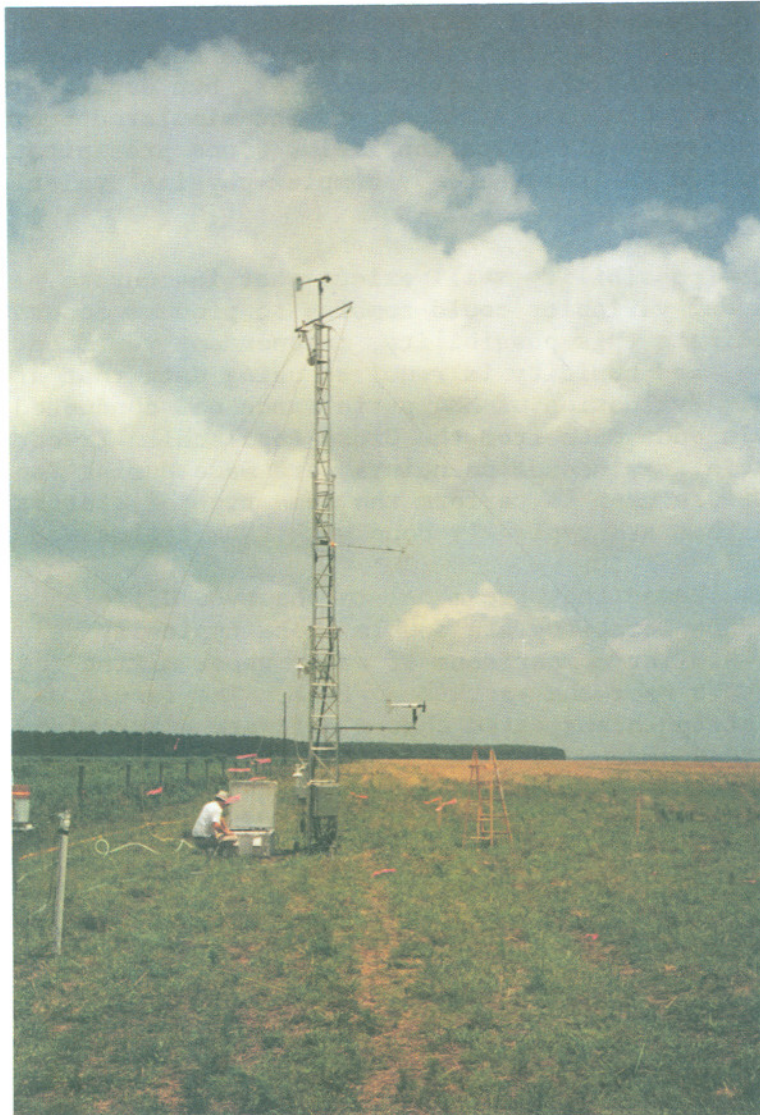
Figure 1. Dry deposition measurement system deployed at the Bondville, Illinois, site.
