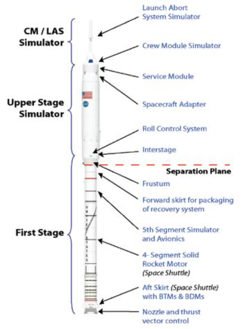
The Ares I-X Flight Test Vehicle will make use of proven space flight hardware.
