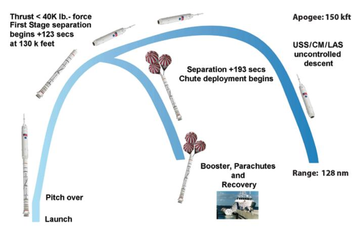
The flight of Ares I-X is designed to simulate the first two minutes of Ares I flight. A broad range of performance data will be relayed to the ground. The solid rocket motor will separate and will be recovered at sea for later inspection. The simulated upper stage and Orion's crew module and launch abort system will not be recovered.
