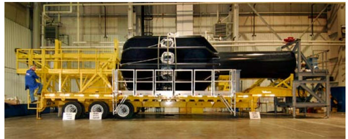
ATK technicians inspect the new Ares I first stage forward casting core for the five-segment booster after delivery to ATK Launch Systems in March 2008. Testing of DM-1 is currently scheduled for April 2009.
