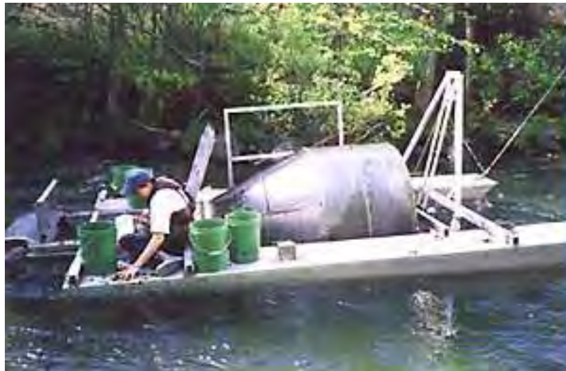
Figure 3-4. The rotary screw trap on Willow Creek, a tributary of Trinity River.
