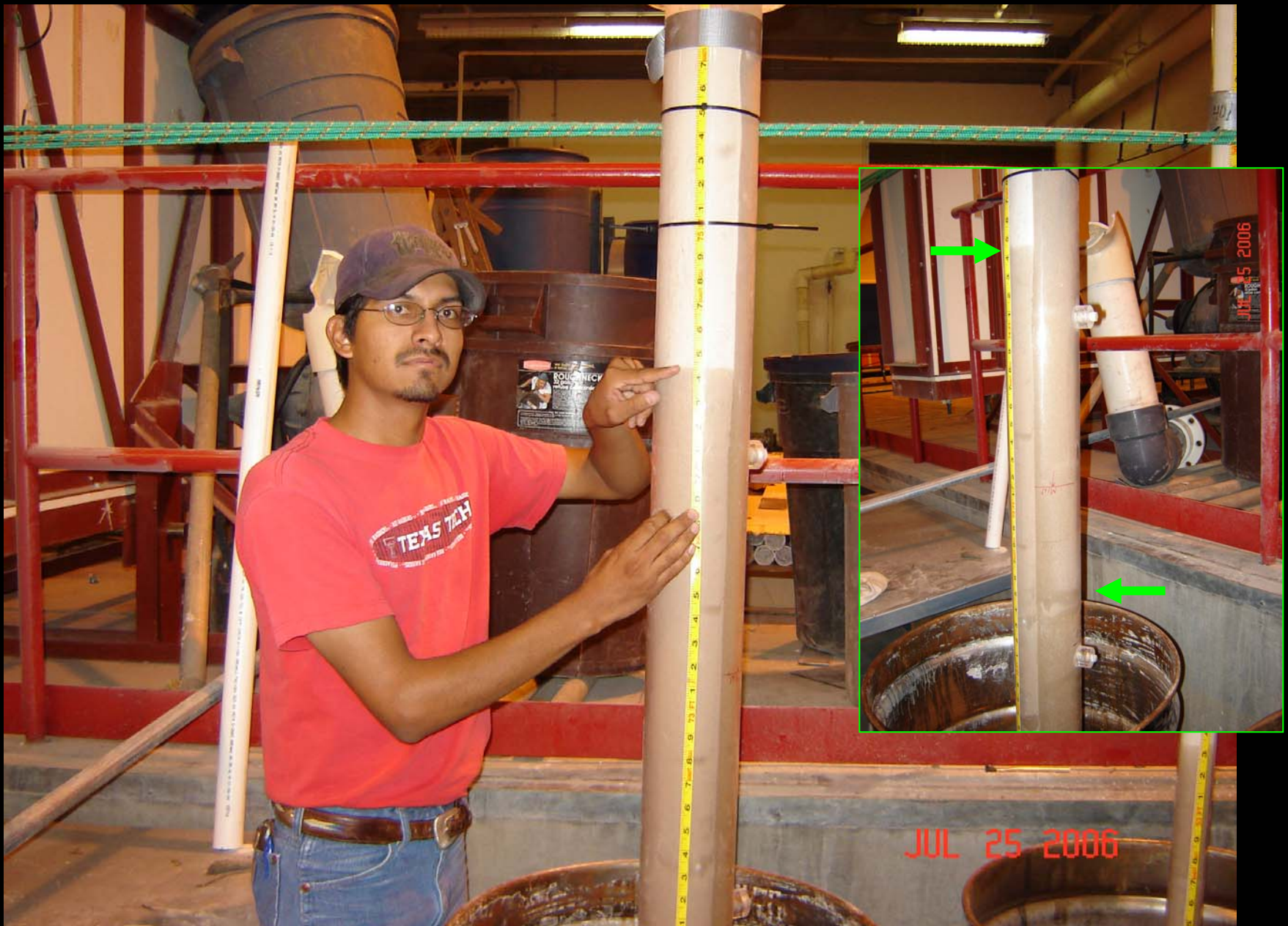
Eric Lopez showing the height of capillary rise in zeolite portion of the 4-inch split sample of zeolite and sand- 2.89 ft (11 days) above water table
