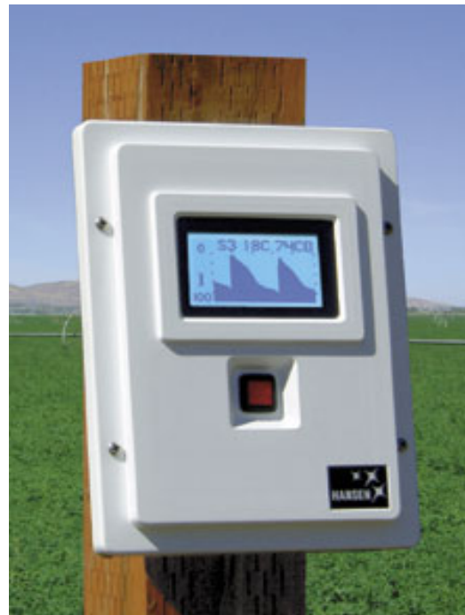
Figure 19, Soil Moisture data recorder with graphing
