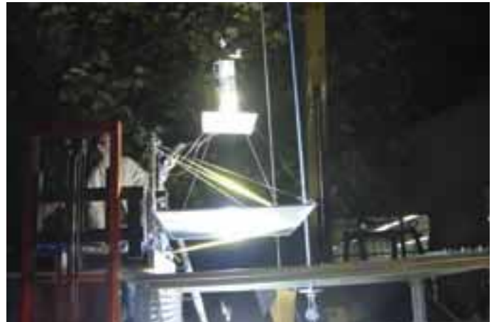
A team demonstrates their concept for a robotic climber that could scale a 200-foot cable powered only by the beam from an industrial searchlight during the 2005 Beam Power Challenge. The challenge was part of NASA's Centennial Challenges. Although none of the 11 teams won the challenge, the University of Saskatchewan Space Design Team had the farthest beam-powered climb, approximately 40 feet. (Photo: NASA/K. Davidian)
