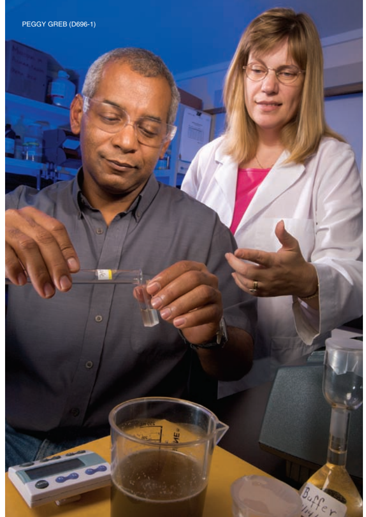
Chemist Gillian Eggleston (right) demonstrates the simple, rapid enzymatic mannitol test to Hedgaro M. Centella, a factory laboratory technician at Alma Sugarcane Factory, Lakeland, Louisiana. A spectrophotometer is required for the test.
