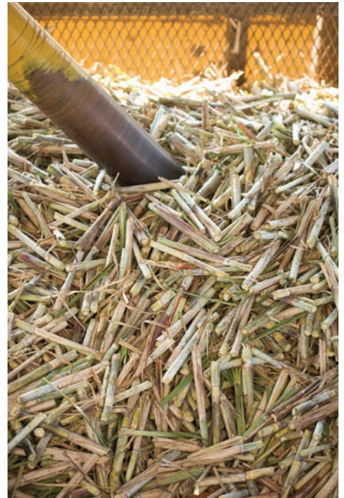
A core press burrows into a shipment of green sugarcane. The sample will be tested for amount of deterioration.
