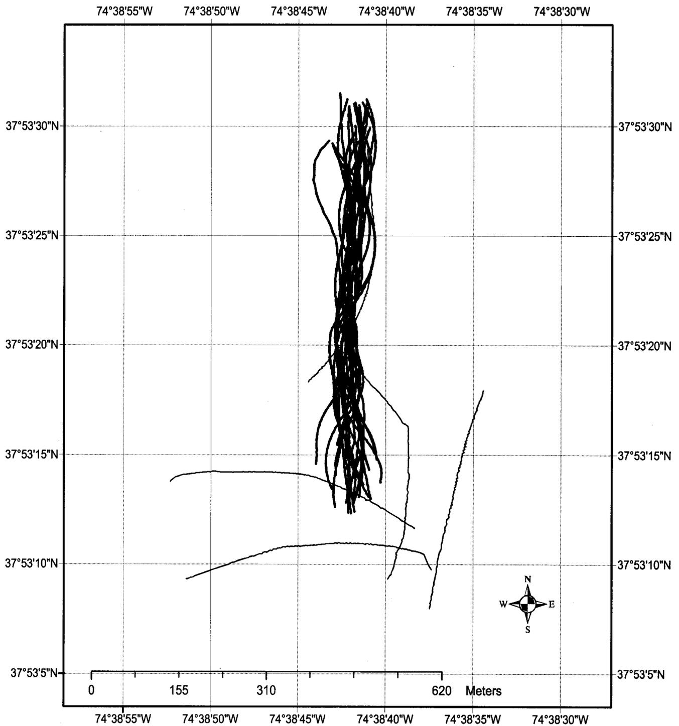
Fig. A30. Towpaths by the *R/V Delaware-II* setup tows (lighter lines) and the *F/V Lisa Kim* (darker lines), 2002, off Delmarva at site: oq02-4.
