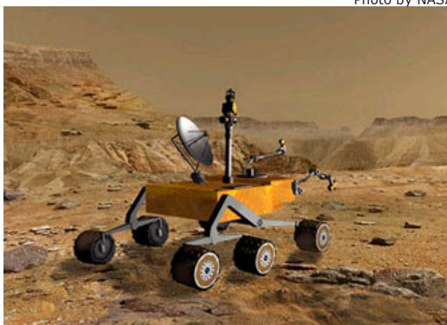
The Mars Science Laboratory will be designed to rove the surface of Mars for an entire Mars year with approximately 10 times the payload mass of the Mars Exploration Rovers
