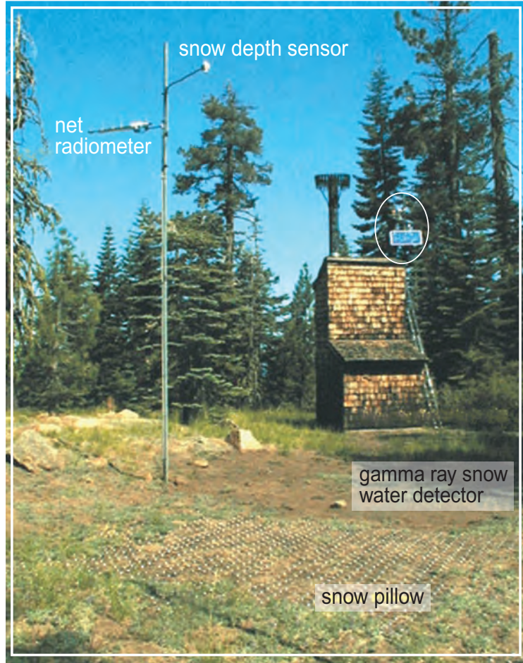
Gin Flat snow-instrumentation site, operated by California Department of Water Resources. Notice Dave Hart, DWR, standing behind and working on the solar panel atop the meteorology/telemetry housing for scale. Photo taken in July 2000.
