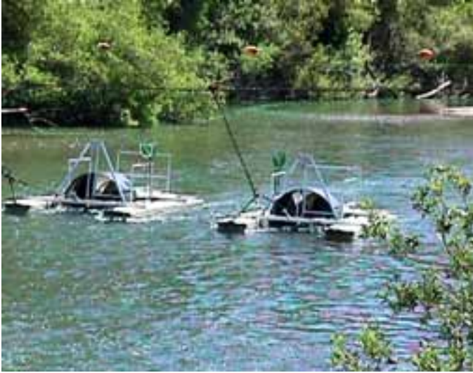
Figure 5. Pontoon rafts with fish counting wheels operating along the Russian River in coastal northern California. Particular attention to fishery habitat is needed when ground water is pumped near streams.
