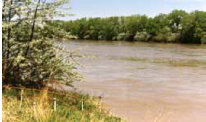
Figure 9. The Rio Grande at Paseo del Norte in northern Albuquerque with three piezometers in the foreground used to monitor shallow, intermediate, and deeper water-levels and temperatures.
