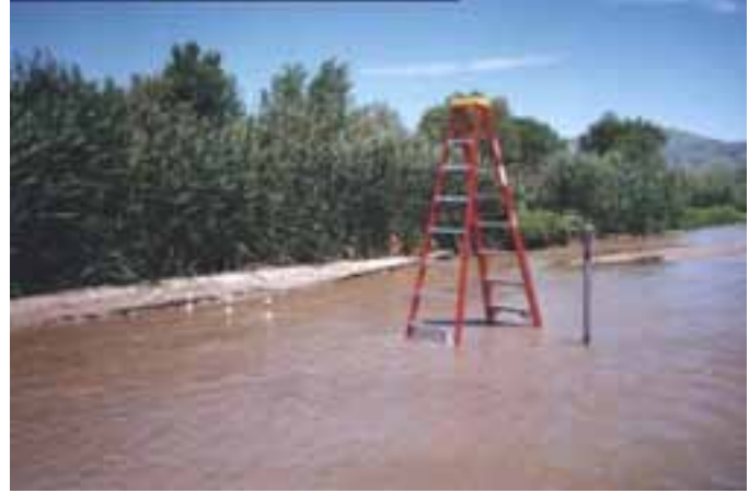
Figure 6. The left photograph shows Site 5 from the north. The right photograph shows a close up of Site 5 with the six small piezometers along side the large piezometer, and the step ladder used to aid in installation.
