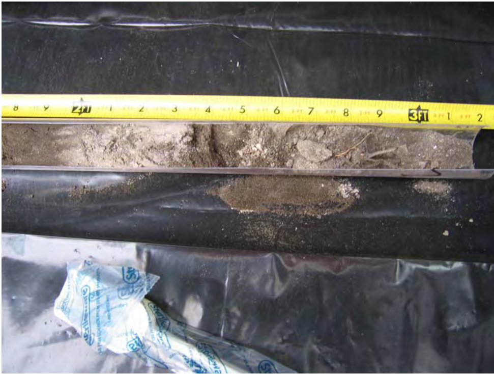
Figure 9: View of “ash-like” substance found at location N6W01-03B. Soil boring interval is from 2.0-2.4 and 2.5-3.0 feet bgs.
