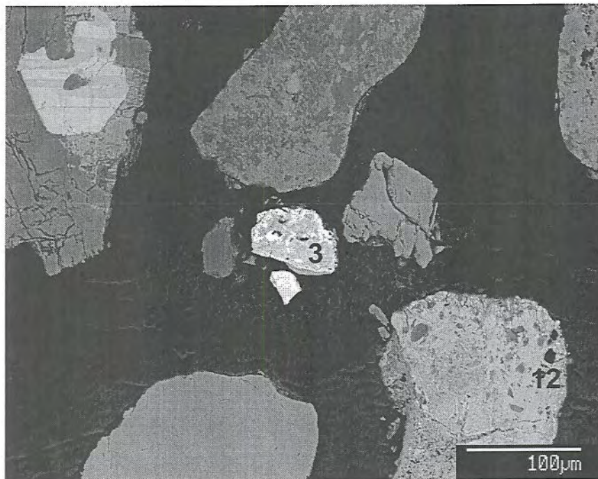
Figure 10. Sample 1 Heavy. Grain at center is an arsenic-bearing iron and lead oxide. Bright particle below it is a zircon and to the right is a spongy, arsenic-bearing iron oxide, likely goethite.
