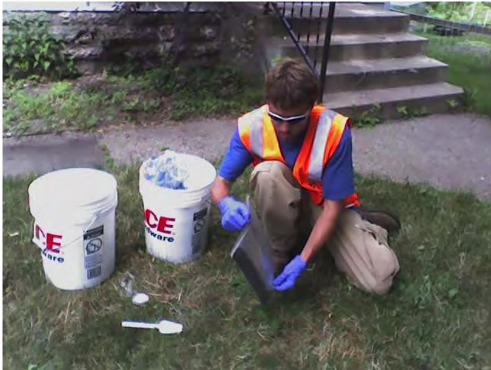
Figures 4 and 5: Typical composite sample homogenization. Soil was placed in the bag from 5 discrete sample locations and homogenized by rotating the bag 15 turns.
