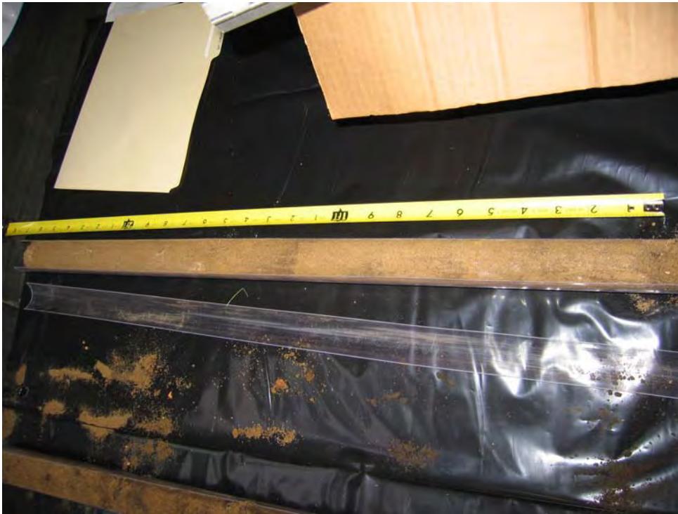
Figure 7: View of soil typically found in lower portion of subsoil (4.0-8.0 feet bgs). Soil description is medium brown to light brown medium to coarse sand with trace gravel, loose, granular structure.
