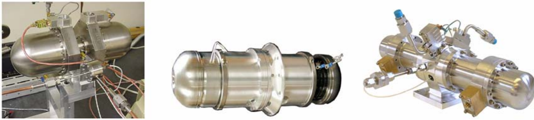
Figure 6-6. Development-Model Cryocoolers from Ball Aerospace, Lockheed Martin, and Northrup-Grumman, at the Time of Testing in 2004
