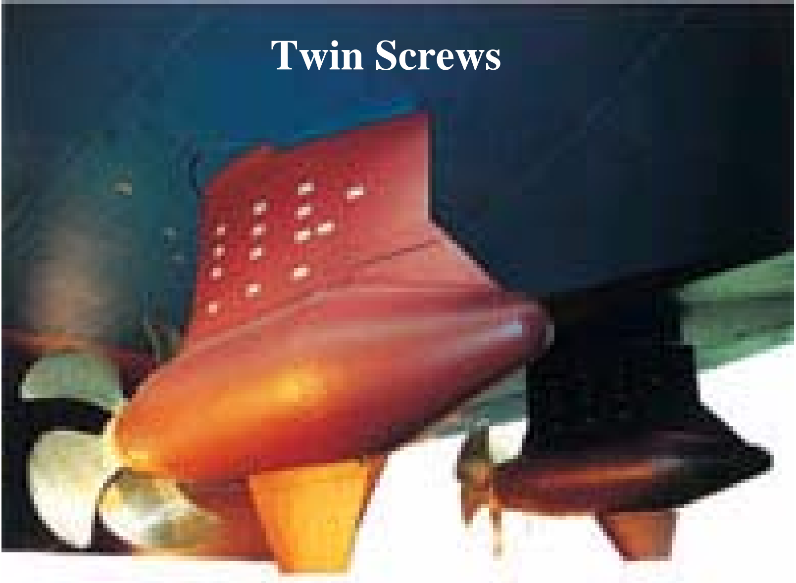
Azipod Trainable “Puller” Props on a Cruise Ship (bow to the left)
