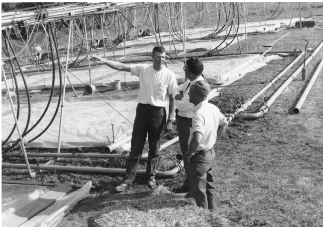
Figure 6. L. Donald Meyer, Agricultural Engineer, National Runoff and Soil Loss Data Center (left) with the “rainulator” set up over erosion plots near West Lafayette, Indiana (circa 1960).
