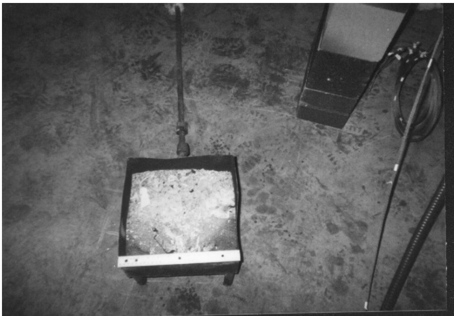
Figure 4-2. Diffusion burner—30 cm × 30 cm (12 in. × 12 in.).
