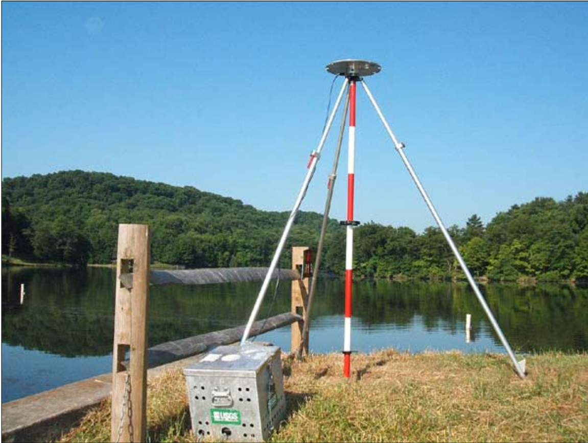
Figure 2. Differential global positioning survey used to establish reference marks near the lake shore.
