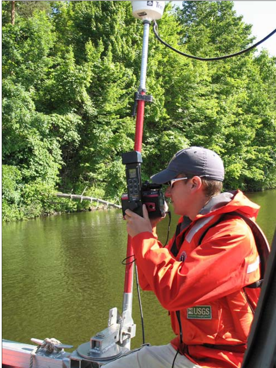
Figure 3. Laser range finder and compass module operated from the transducer and differential global position system location to define the shoreline.
