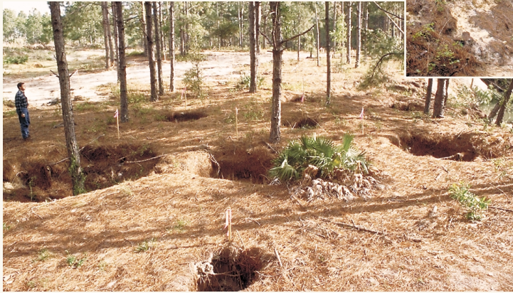
Sinkholes induced during the development of an irrigation well affected a 20-acre area and ranged in size from less than 1 foot to more than 150 feet in diameter.
