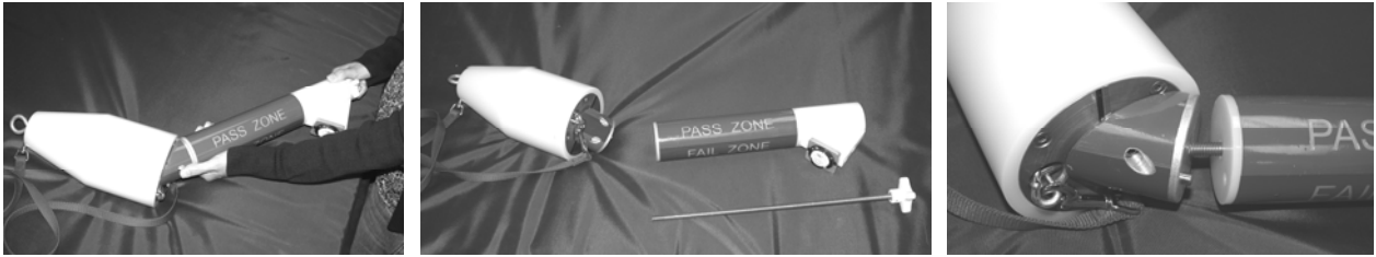
Figure 6. Disassembly and assembly of the cone and cylinder tool.
