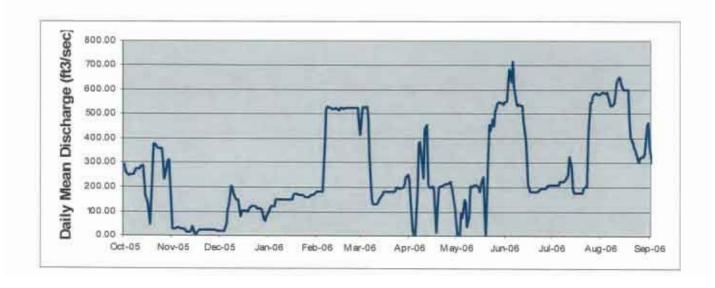
Location. —Lat 40°25'02', long 105°14'35', Larimer County, Hydrologic Unit 10190006, 11 miles west of Loveland, Colorado, on the Big Thompson River. Gage. — Water-stage recorder with satellite telemetry at Parshall Flume. Elevation of gage is 5520 feet from topographic map.
