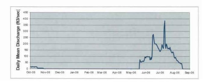
Location. —Lat 40°25'16', long 105°13'26', Larimer County, Hydrologic Unit 10190006, 9 miles west of Loveland, Colorado, on the Big Thompson River. Gage.—Flow meter with satellite telemetry. Elevation of gage is 5280 feet from topographic map.
