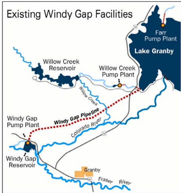
Figure ES-1. Windy Gap Reservoir facilities.
